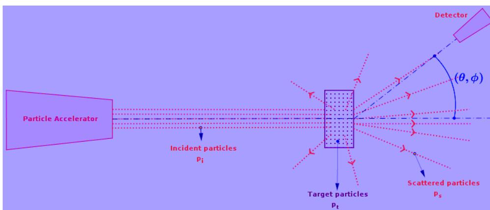
Figure 2.4: Schematic diagram of a scattering experiment. The particle accelerator is on the left, target in the middle, and detector on the right. Source: Design generated using Geogebra software
