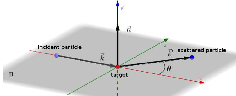
Figure 2.7: Scattering plane is spanned by the initial and final wave-vectors  $\vec{k}$  and  $\vec{k}'$ . Source: Drawn using Geogebra Software
